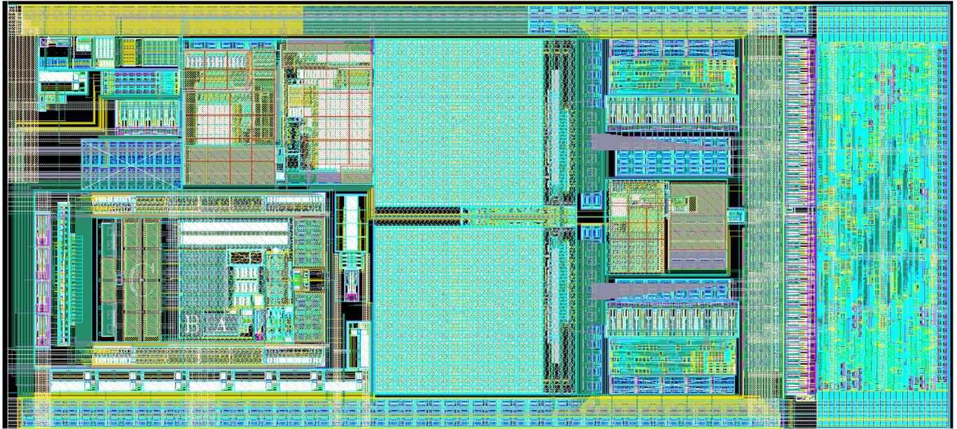
Figure 6:ADC top level layout
