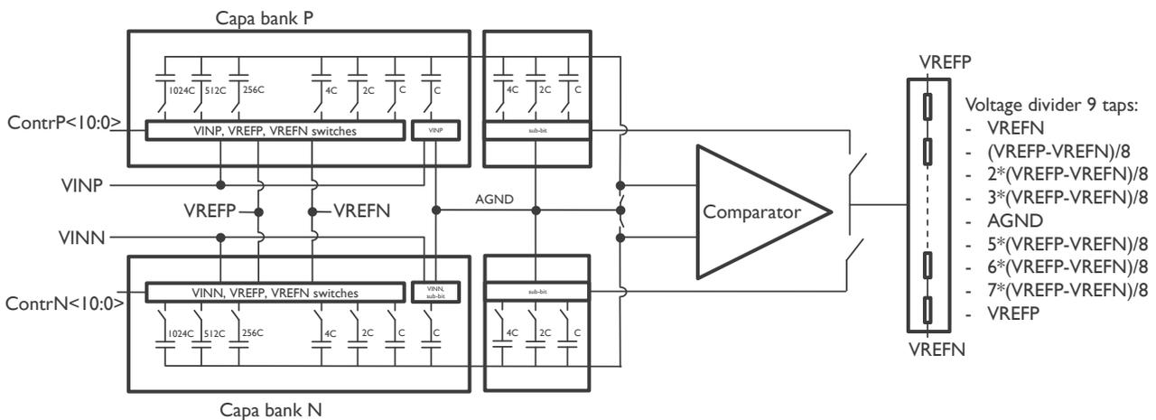
Figure 5: Improved 14 bit DAC for ADC DAC
