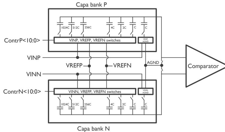
Figure 4: Original 11 bit DAC for ADC
