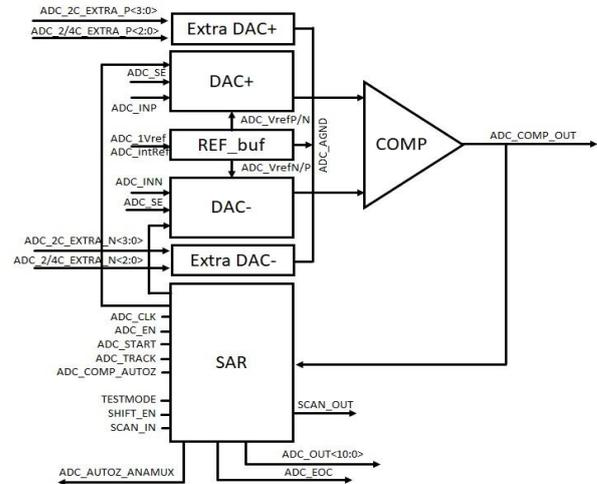
Figure 3: Block diagram of ADC Core
