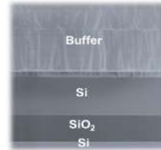
TEM cross-section of GaN/AlGaIn superlattice-based buffer on SOI substrate.
