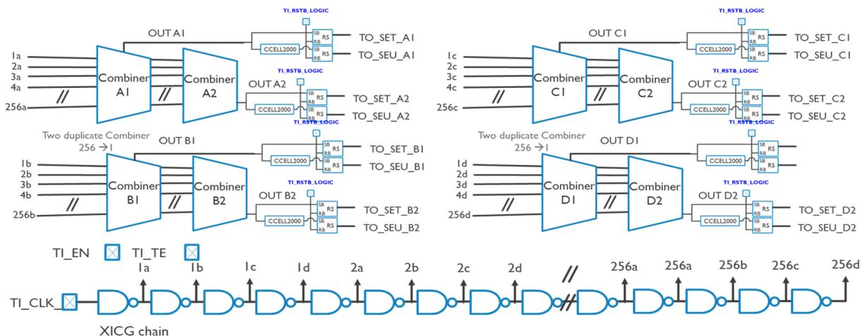
Figure III-2 SET/SEU test structure for clock gating cells
