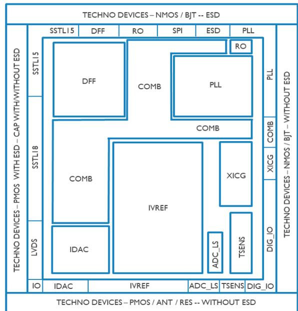
Figure II-1 Abstract floorplan of the test vehicle
