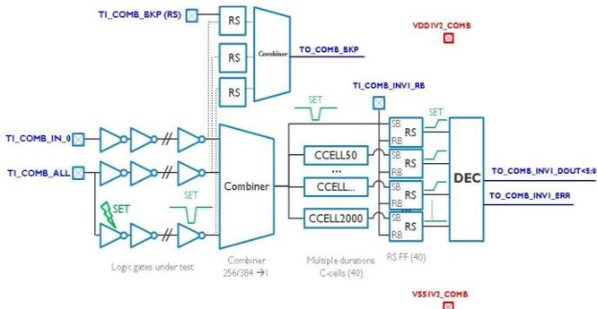
Figure III-1 SET test structure for combinatorial cells
