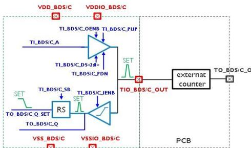
Figure III-3 Test structure for digital IOs
