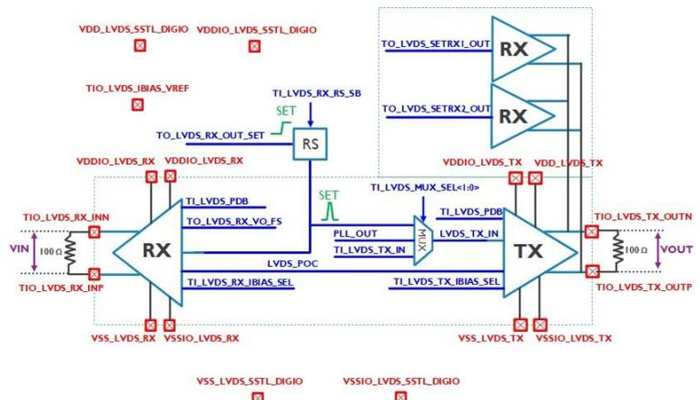
Figure III-4 SET test structure for LVDS
