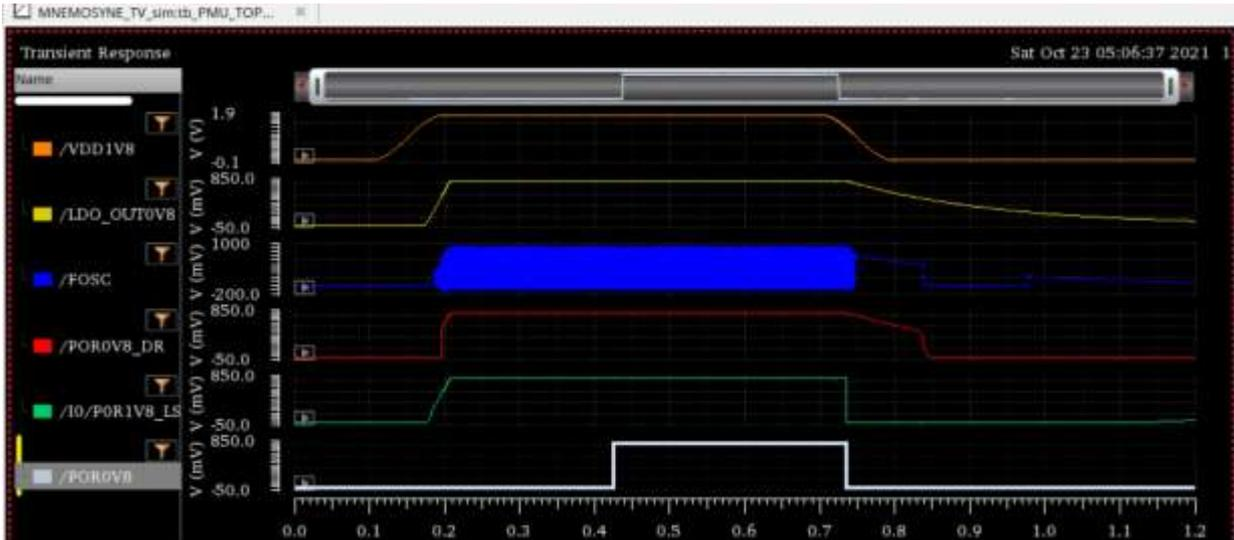
Figure 3: Essential PMU power-up and power-down. The digital delay using the oscillator ensures that the reset is released only after a safety interval of few 100usec.
