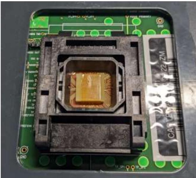
Figure 9: Test board with socket
