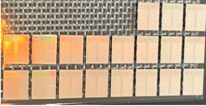
Figure 7: First set of test vehicle dies before assembly
