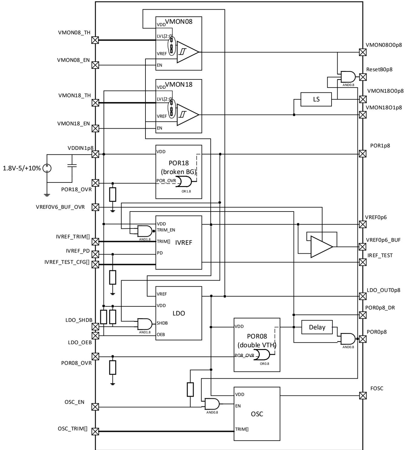
Figure 2: High level view of PMU
