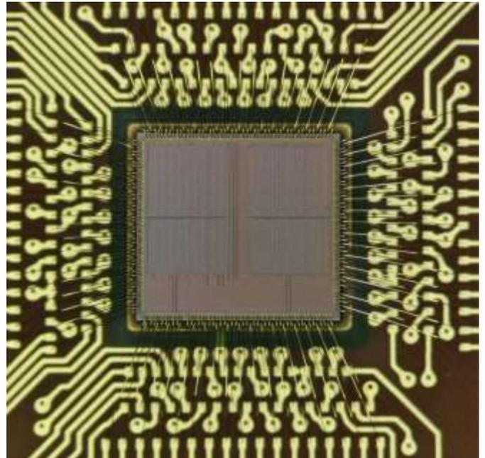
Figure 1: Test Vehicle bonded to substrate.
