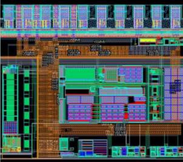
Figure 5: PMU layout with clearly visible LDO bond pads along the north edge, oscillator to the west, IVref in the east PORs, VMONs and glue logic in the south.
