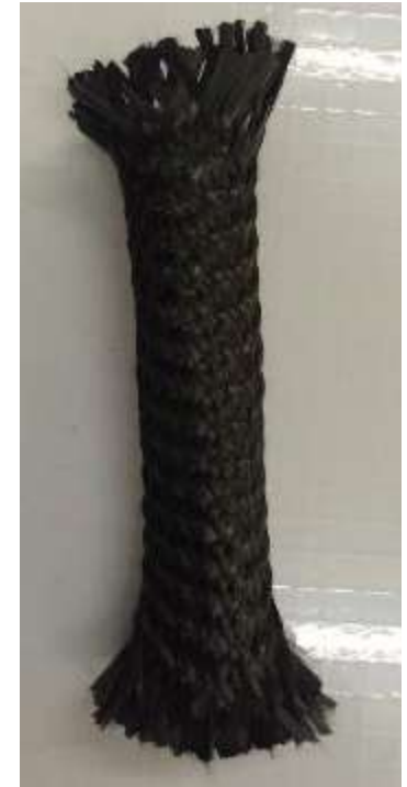
3 D interlocked Braided carbon fiber structure
