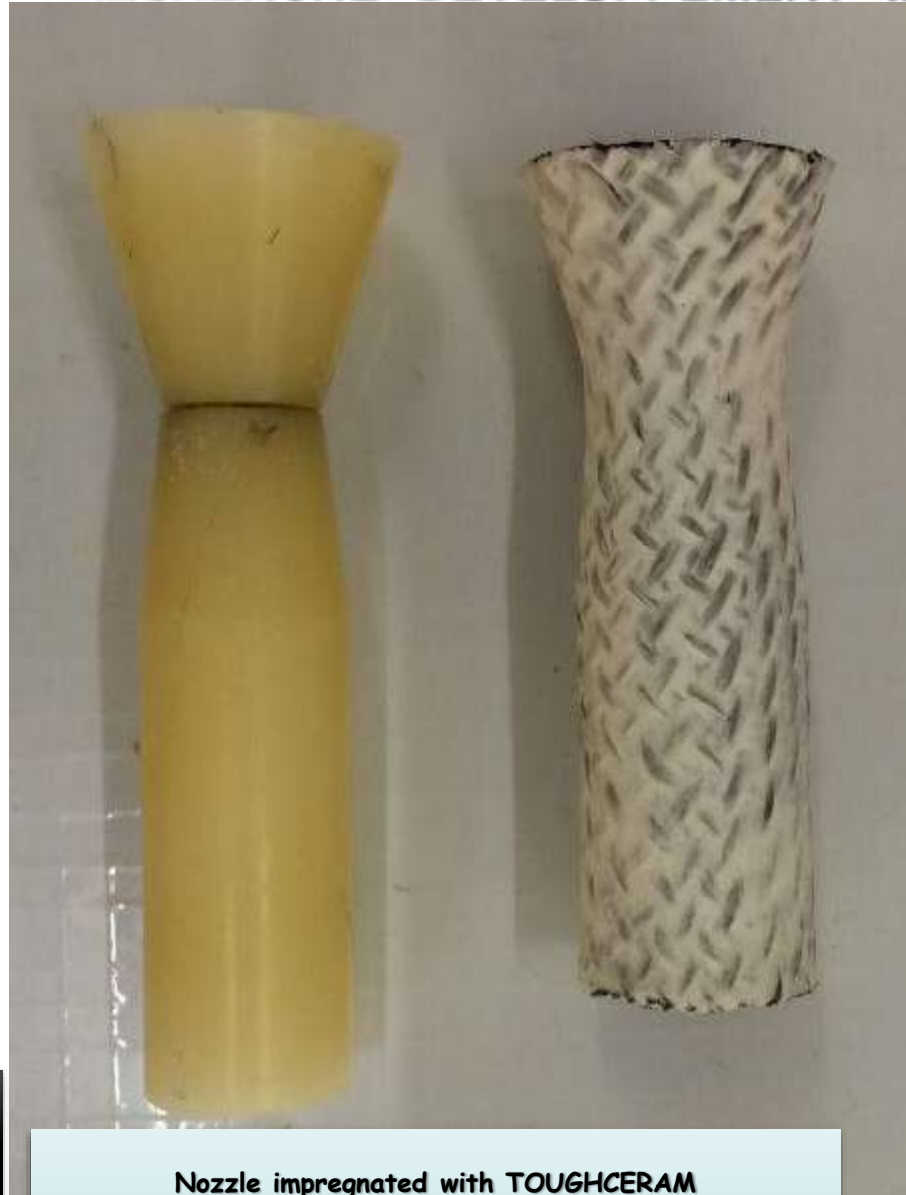
Nozzle impregnated with TOUGH CERAM ceramized @ 1100°C
