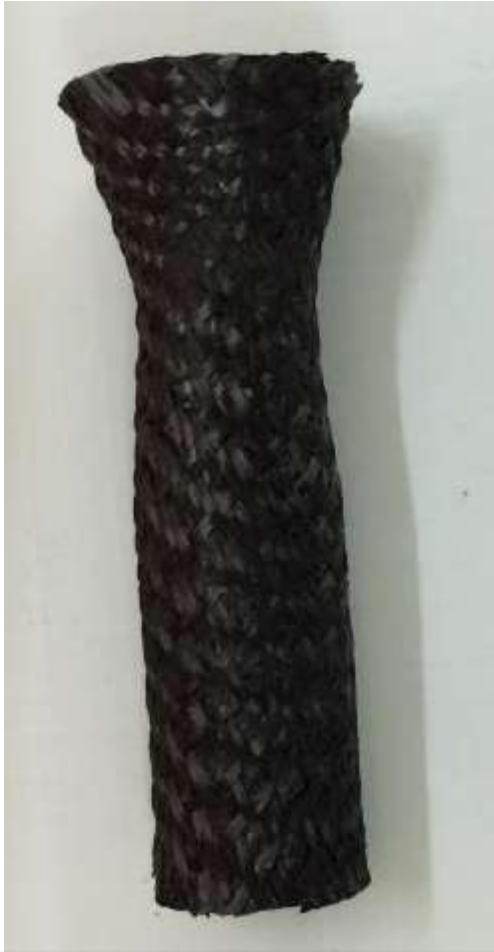
Nozzle impregnated with TOUGH CERAM ceramized @ 1100°C
