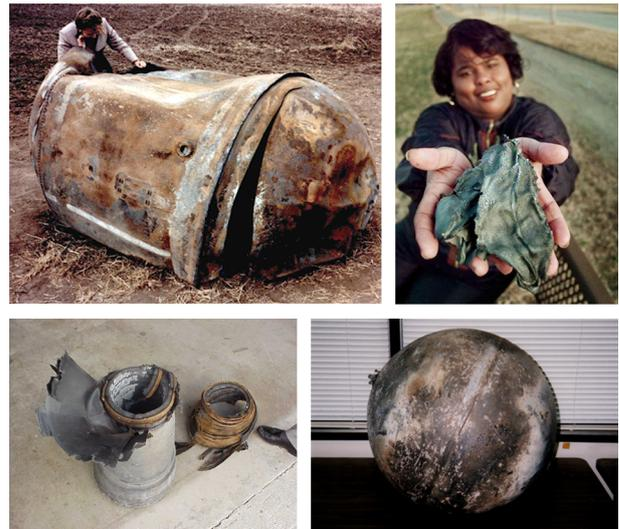
Figure 1. Delta-II Second Stage - Recovered Fragments (Credit: NASA, Tulsa World, Aerojet)
