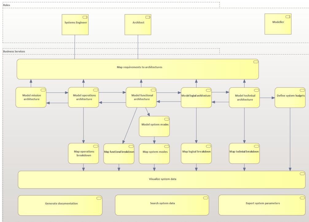
The extended MBSE environment for system architecting hosts interacting MBSE services that serve the main MBSE processes to generate consistent mission and system architectures.
