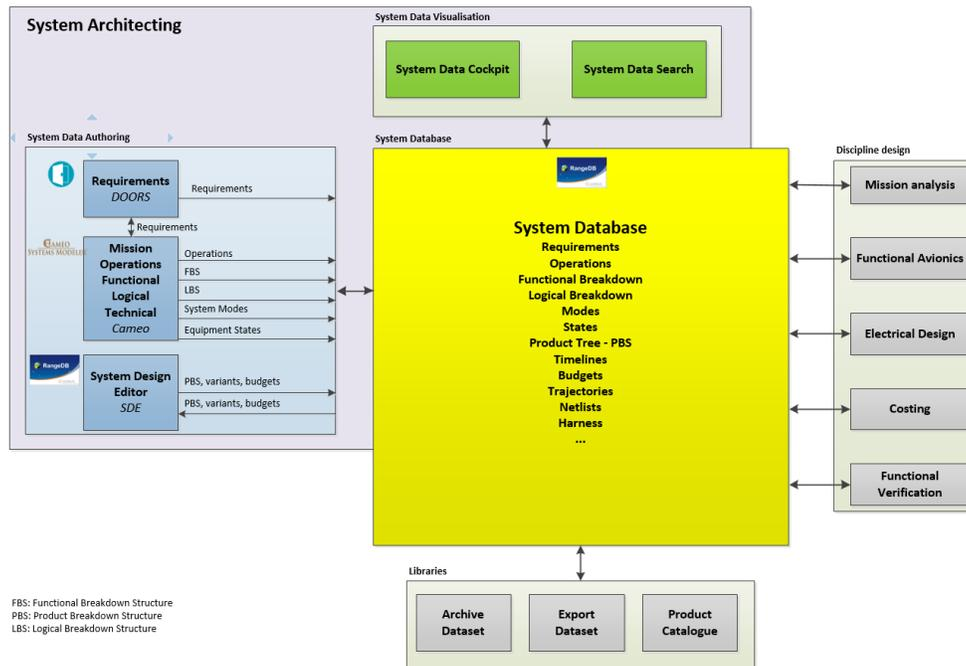
The extended MBSE environment for system architecting allows defining, maintaining and exchanging the system data in specific authoring tools. This is mainly relying on the system database, interfacing the requirements database (DOORS) and the architecture definition database (Teamwork Cloud).
