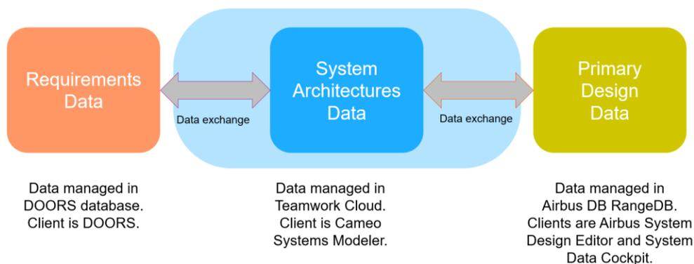
The main motivation is to build the Mission, Operations, Functional, Logical and Technical architectures that are consistent and well aligned with the Requirements and the System Preliminary Design.
