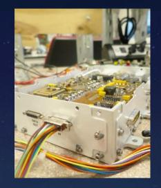
Used for the remote safe ignition of pyrotechnical chains. The system is particularly indicated for solid rocket motor ignition.
