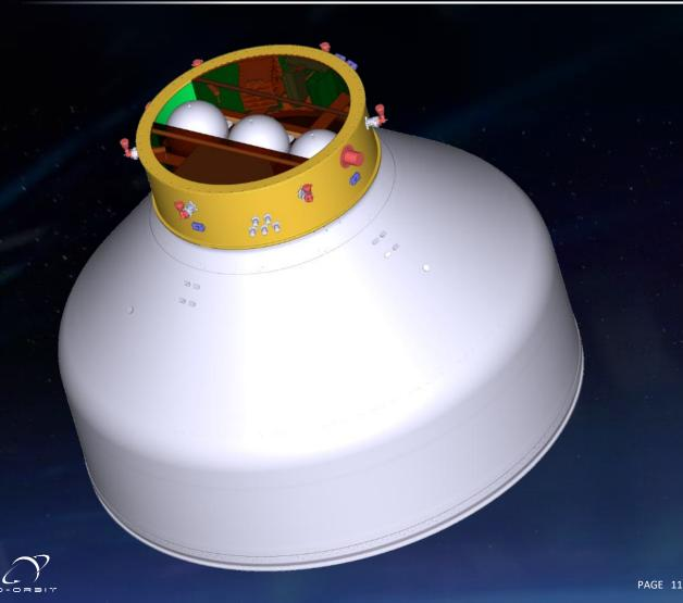
The deorbiting kit is a cylinder of customizable diameter and height. The IOD is 1100mm diameter by 300mm diameter, and only includes:
