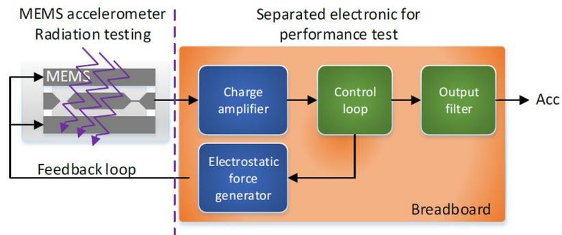
Figure 6: Radiation testing of the MEMS accelerometer only
