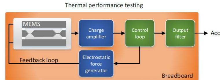
Figure 7: Accelerometer breadboard with individual package MEMS sensor and discrete electronic components
