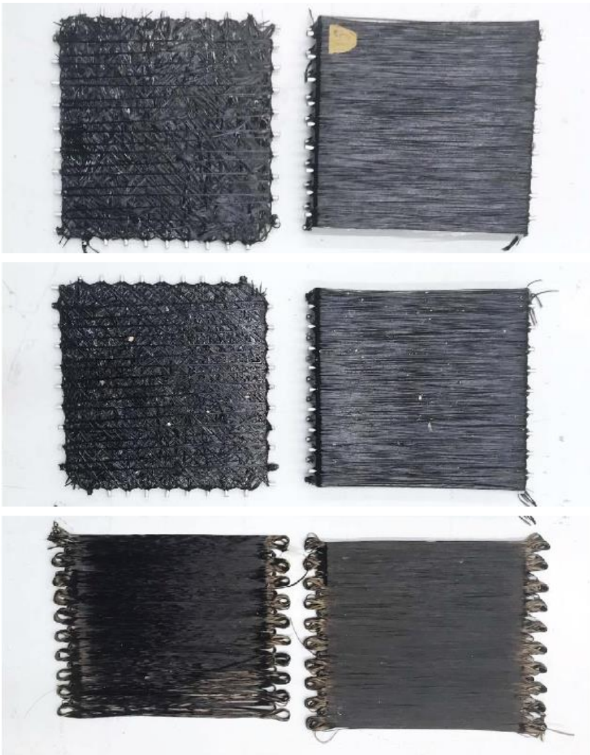
Mechanical samples produced with two different fibre layouts:
