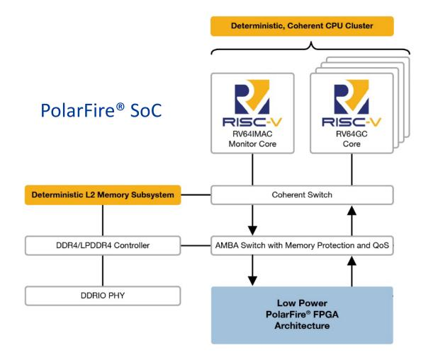
Asymmetric processing with 2X power efficiency Quad-core 64-bit RISC-V processors Linux<sup>®</sup> and Real-time operating systems Highly flexible 2MB L2 cache
