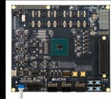
Lattice Evaluation board Easy access to I/O and SerDes
