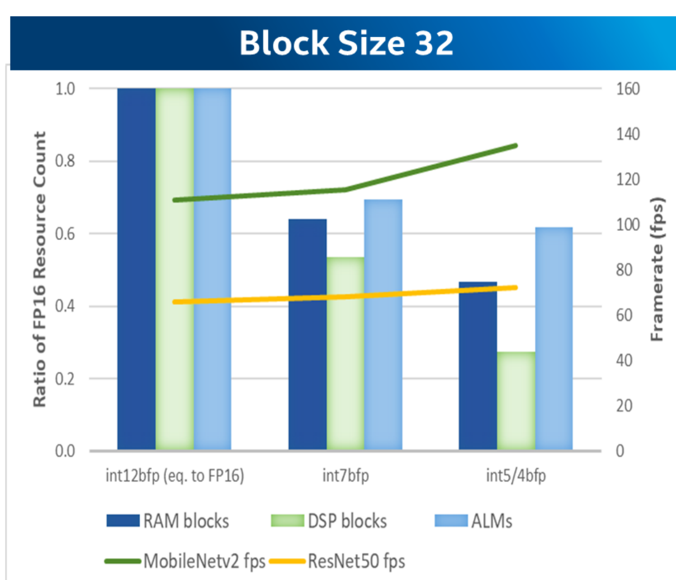
Resource count ratios and framerate for ResNet 50 and MobileNet v2 inference at block size 32 on Arria® 10
