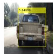
Vehicle Detection Using YOLO v2 Deployed to FPGA
