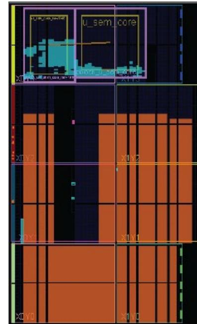
Figure above shows implementation of full-protected snake architecture
