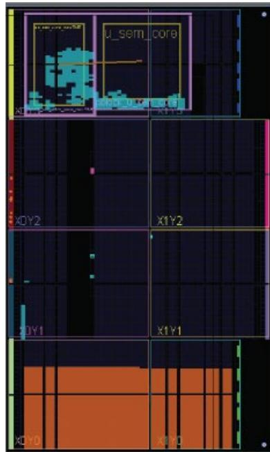
Figure above shows a floorplan in Artix-7 when non-protected Snake architecture RTL is implemented
