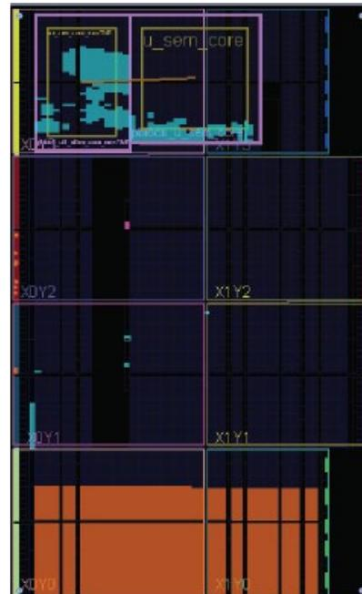
Figure above shows a floorplan in Artix-7 when partial-protected
