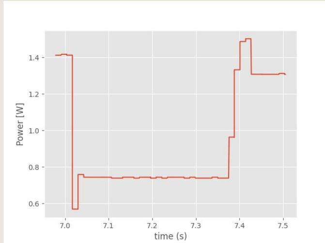
Graph shows the profile of power consumption during reconfiguring the FPGA
