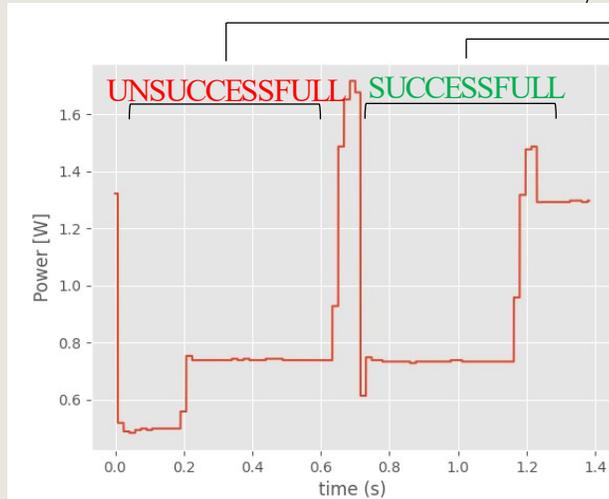
Graph shows the profile of power consumption during unsuccessful reconfiguration and followed by successful FPGA reconfiguration.
