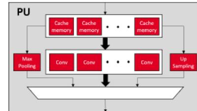
Figure 6: Block diagram of the Processing Unit
