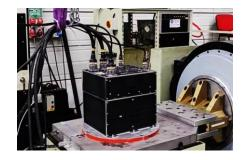
Electronics Racks for Shock & Vibration
