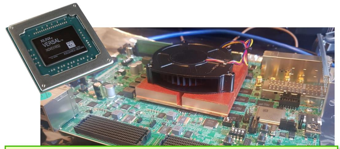
A quick look at the Versal Evaluation Board clearly shows that this board is far away from a Space board, so when a new FPGA is introduced, a lot of steps are needed to assess how to use it for Space application. Topics such as package, assembly, power supply, boot, thermal dissipation, complexity of board place and route, knowledge of radiation effects, etc... shall be considered.
