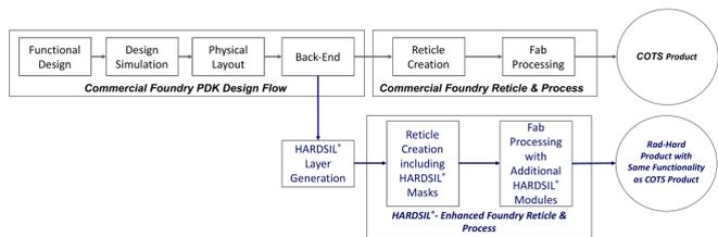
Figure 6: Example High-Level IC creation flow showing the use of the same design infrastructure to create both standard commercial and rad-hard products and the ability to manufacture the same IC in both commercial and rad-hard versions
