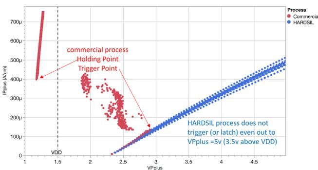
Figure 4: Typical Latch-Up for Commercial and HARDSIL<sup>®</sup> Enhanced Process at 300 K
