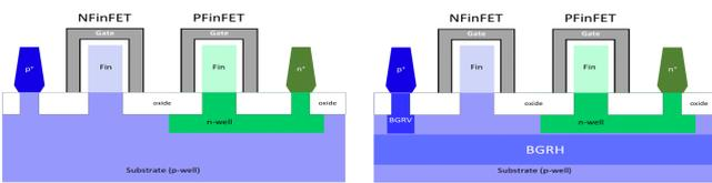
Figure 2: Commercial vs. HARDSIL<sup>®</sup> for FinFET Processes
