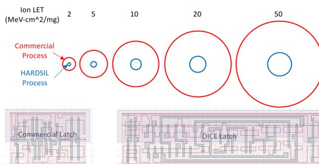
Figure 3: Particle Strike Upset Region vs. Process by Ion LET Compared to Latch Cell Areas
