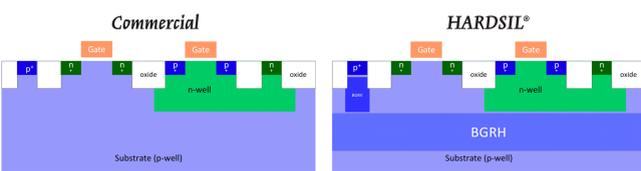
Figure 1: Commercial vs. HARDSIL<sup>®</sup> for Horizontal Processes
