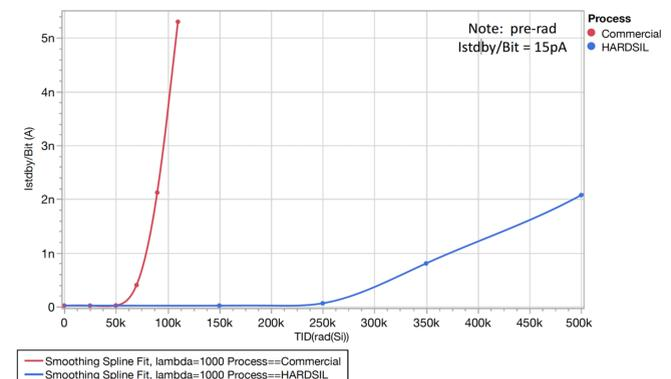
Figure 5: Typical Standby per Bit vs. TID for Commercial and HARDSIL<sup>®</sup> Enhanced Devices
