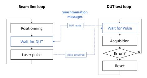
Fig. 6.3: Scan Mode C: Synchronous test
