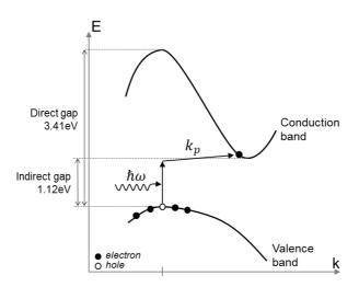
Fig. 3.3: simplified band diagram of silicon and principle of phonon-assisted indirect band-to-band absorption of a photon by an electron
