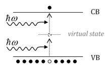
Fig. 3.6: principle of the Two Photon Absorption process
