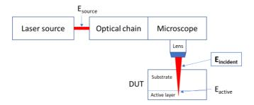
Fig. 7.1: Different laser pulse energy definitions
