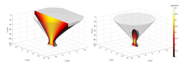
Fig. 5.1: Typical SPA (left) and TPA (right) induced charge distribution in a 100μm Si substrate
