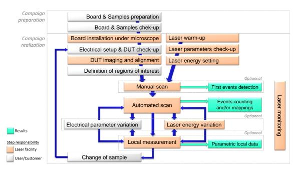
Fig. 3.9: main steps of a typical laser testing campaign
