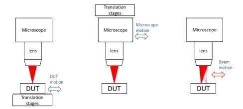
Fig. 6.2: different implementations of the scanning motion: DUT motion (left), Microscope motion (center),
