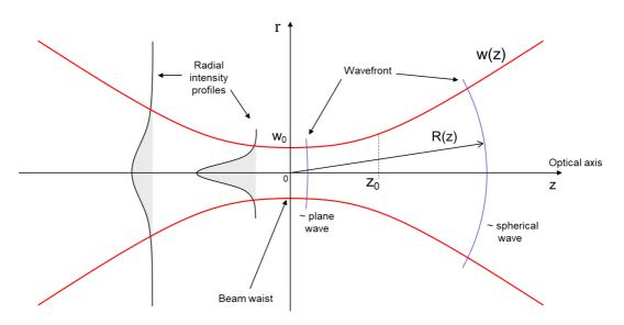
Fig. 3.1: schematic definition of a Gaussian laser beam
