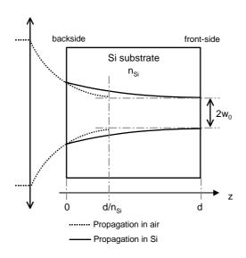
Fig. 3.2: effect of the refraction index on beam focusing through the substrate
