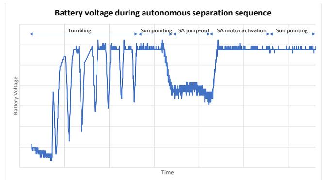
Figure 4: Battery voltage during execution of autonomous separation sequence, MTG-I1, 13th of December 2022
