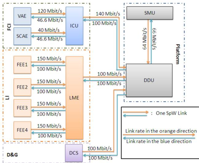
Figure 2: SpaceWire network on MTG-I
