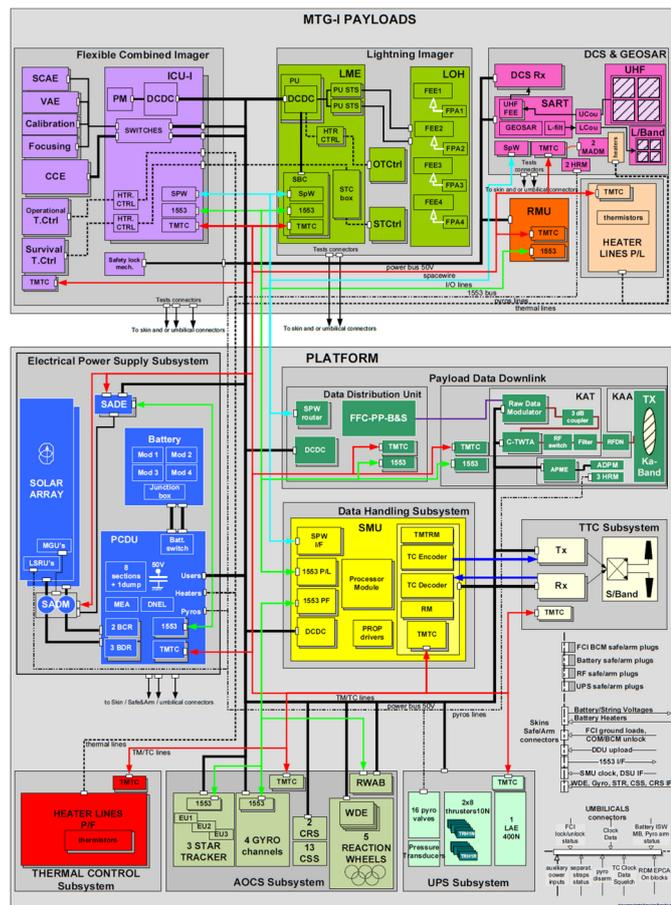
Figure 1: MTG-I satellite data handling architecture
