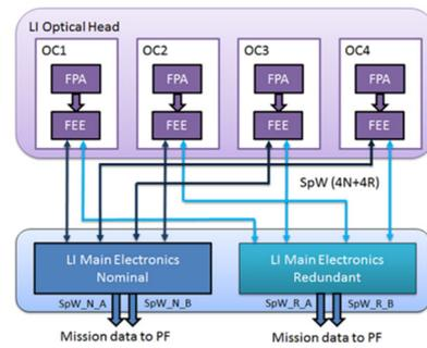
Figure 3: LI SpW internal network
