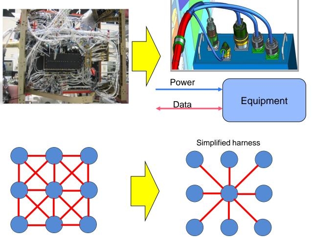
Reduction of interfaces and thus simplification of harness topology with reduced connections
