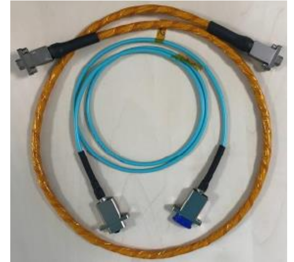
SpaceWire in orange Vs Multi-fiber cable in blue (courtesy of Axon)
