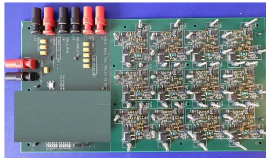
POLLUX Automated test bench
