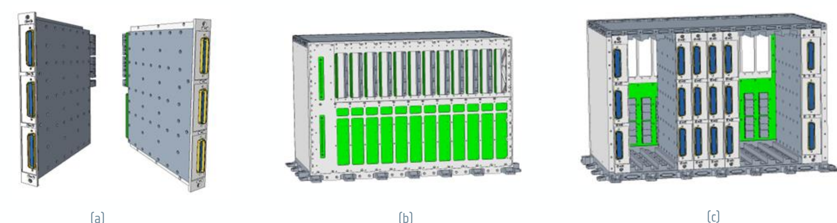
Figure 3: Preliminary Renderings of ADHA module (a), ADHA unit with EMC cover (b), and fitted ADHA unit with modules (c), taken from [AD014]
