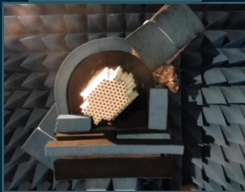
LEO active antenna demonstrator during antenna test (Courtesy Airbus Defence and Space).
