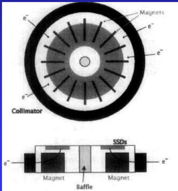
The Miniaturized Electron Magnetic Spectrometer (MEMS) was designed to measure 0.05 - 1.5 MeV electrons using PSD along a  $360^\circ$  range of azimuth angles.
