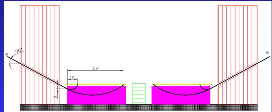
2 kGauss bend up to 2 MeV electrons onto the PSD, when the incidence angle is  $60^\circ$  wrt instrument axis.
