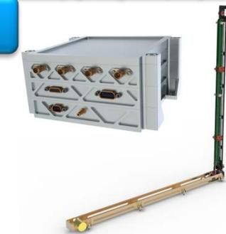
Multi-Needle Langmuir Probe (M-NLP) [Eidel, No]
