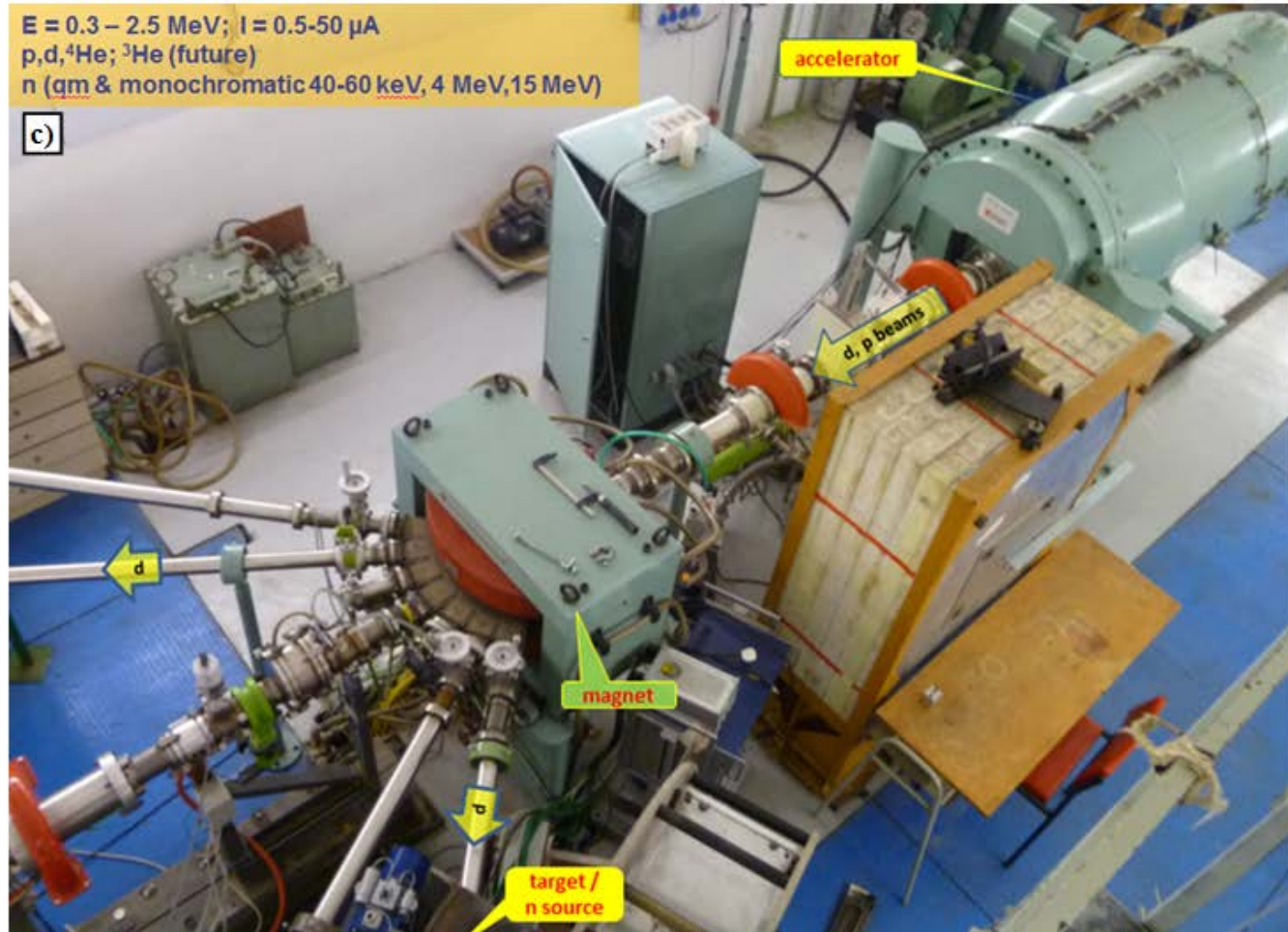
Clean room (a), X-ray \mu -imaging & \mu -tomography unit, X-ray pencil beam test bench (b), Van de Graaff accelerator, beam guides (c).
