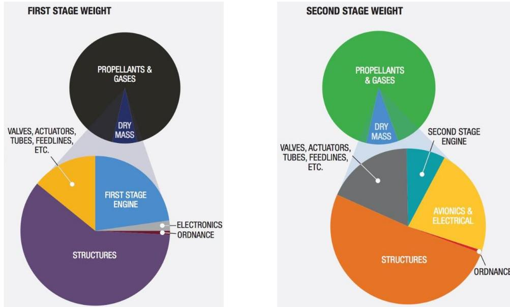
Fig. 7: Subsystem weight distribution for core and upper stage [3]
