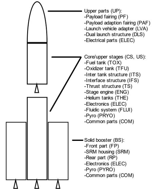
Fig. 8: Subsystems data provided by ArianeGroup
