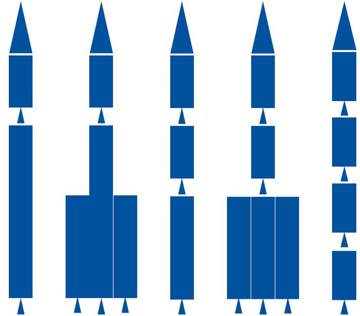
Fig. 5: Different tandem and parallel staging concepts
