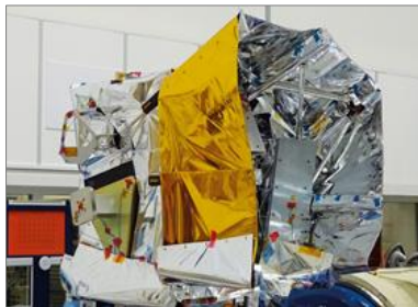
Thermal H/W (Radiators, Thermal Straps, MLI, etc)
