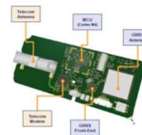
• Syntony prototype (as an example, to implement SoftSpot IoT)
