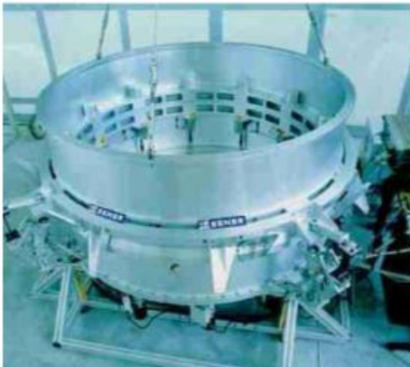
Docking/Berthing (COLUMBUS/HERMES); International Docking & Berthing Mechanism (IBDM).
