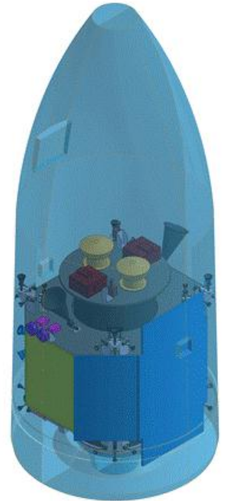
Vega physical accommodation
