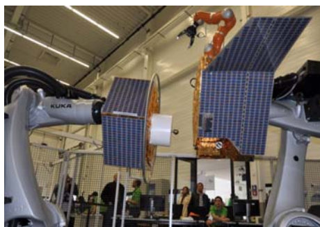
DEOS-Simulator Test setup for grasping and manipulation
