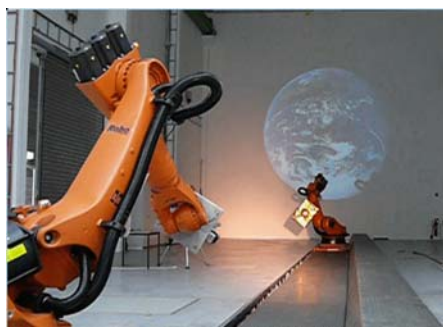
EPOS Test setup for approaching and docking
