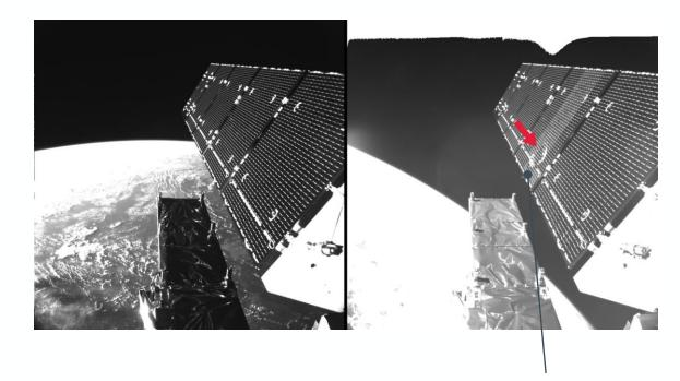
hit by ~5mm debris in 2016, resulting in 40 cm damage and at least 8 trackable debris (> 5cm)
