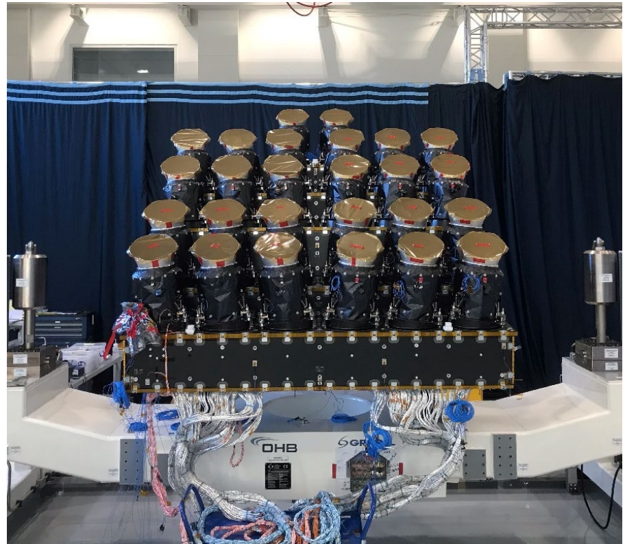
Cameras on optical bench (Mechanical-Therma-Dummies)
