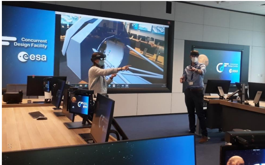
Figure 1 Two users running a design exercise with ARCE at the CDF, ESTEC, and moving pieces of the 3D model while the presentation mode is active and visible on the projector canvas
