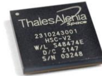
Figure 2: HSC PBGA package for Space applications
