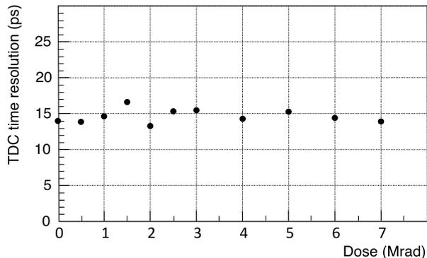
Fig. 3 - TDC time resolution as a function of TID measured with TOFHIR2 [10].
