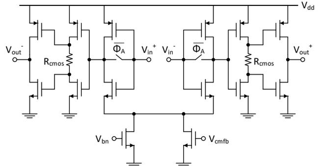
Figure 2 - Proposed ring amplifier, derived from [11].
