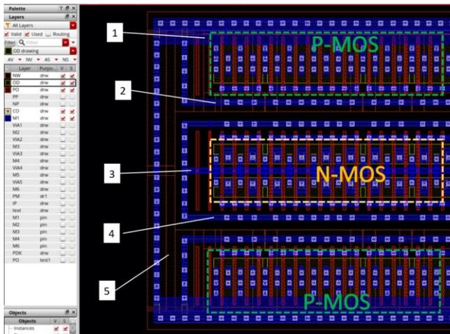
Figure 5 - Layout approach used to improve circuit robustness to latch-up due to radiation.
