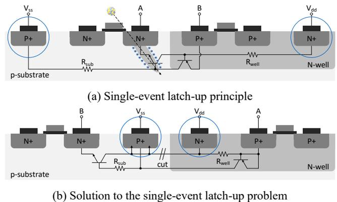
Figure 4 - Single-event latch-up principle and solution [12].
