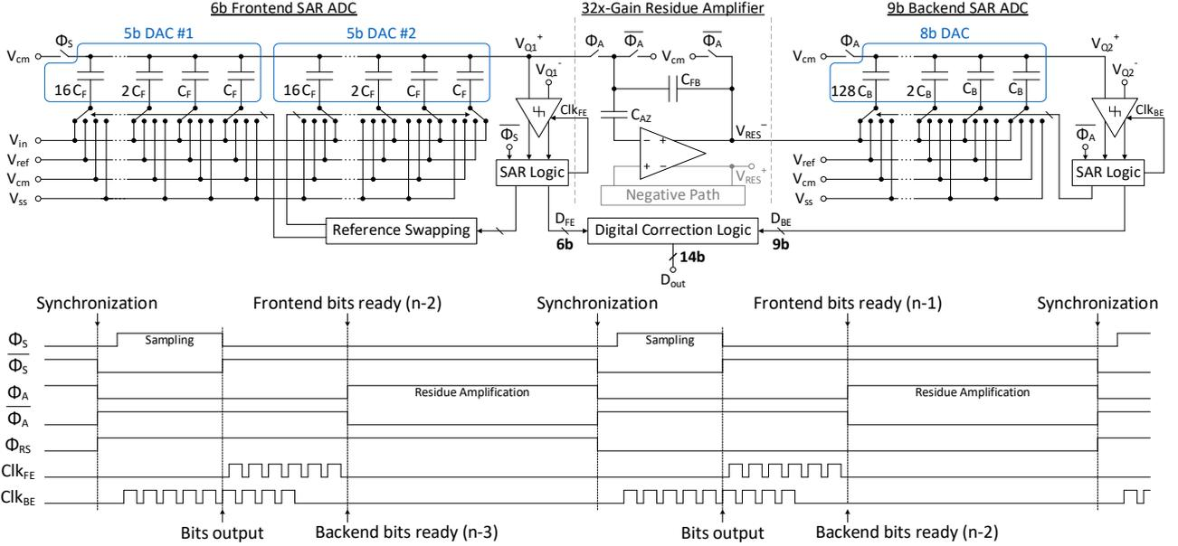
Figure 1 - Proposed 14-bit 80 MS/s pipeline SAR ADC.
