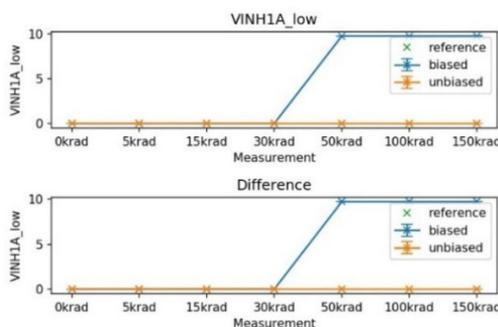
Fig. 5. Drift of open drain output voltage of RUCA1 during TID in Volts.
