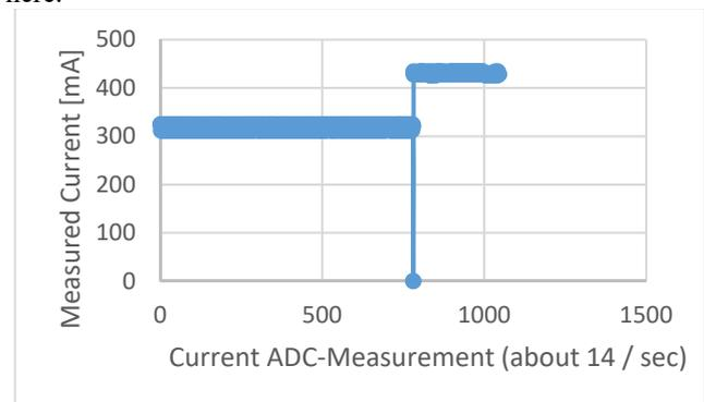
Fig. 7. Main Supply Current of Device 15 During a latch-up test at Xenon. Current is measured via an ADC at an external sensing resistor.
