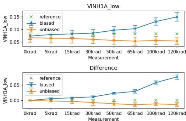
Fig. 11. Drift of RUCA2 open drain output voltage vs. TID in Volts
