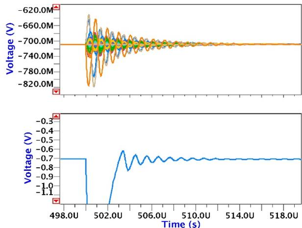
Fig. 9. Simulation results of VGATE when different nodes are hit by single event pulse during simulation
