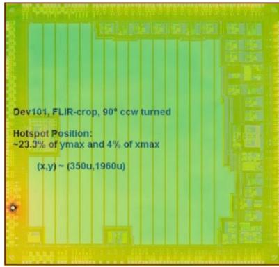
Fig. 10. RUCA1 FLIR-Investigation showing hot spot in IO-Ring
