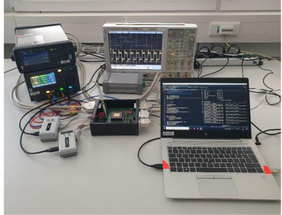
Fig. 3. Measurement setup for RUCA TID measurement campaign
