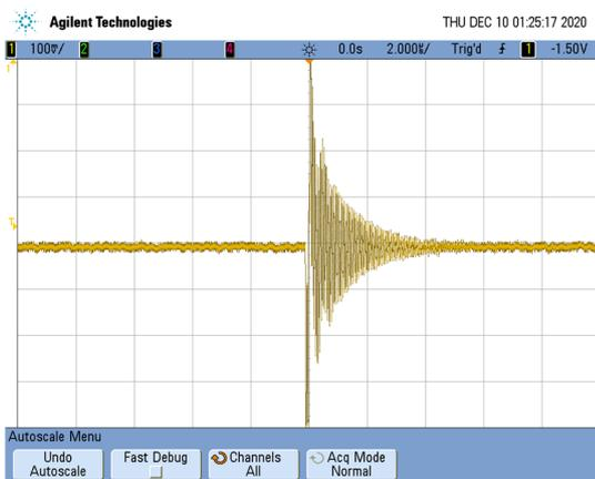
Fig. 8. Measurement result of VGATE from first RUCA1 SEE Campaign at 32 MeVcm<sup>2</sup>/mg
