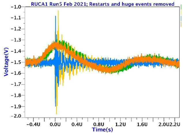
Fig. 6. RUCA1: DAC2 for 45.8 MeVcm<sup>2</sup>/mg. Results of a single run overlaid. x-axis in seconds, y-axis in volts. Maximum amplitude is about 450 mV for fast oscillations and about 210 for slow. Restarts and huge events have been removed as they are not DAC related
