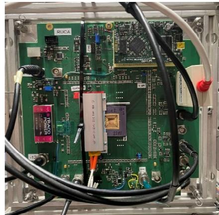
Fig. 4. RUCA2 Radiation test setup mounted in chamber at HIF of UCL
