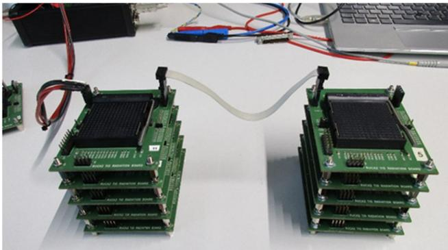
Fig. 2. Stacked irradiation boards for total dose tests of RUCA
