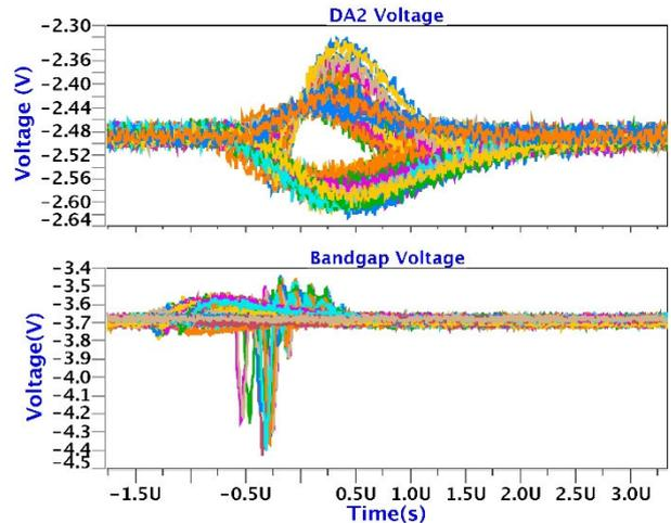
Fig. 12. RUCA2: DAC2 (top) and Bandgap voltage, for 45.8 MeVcm<sup>2</sup>/mg. Results of all devices overlaid. x-axis in seconds, y-axis in volts. Maximum Amplitude is about 165 mV
