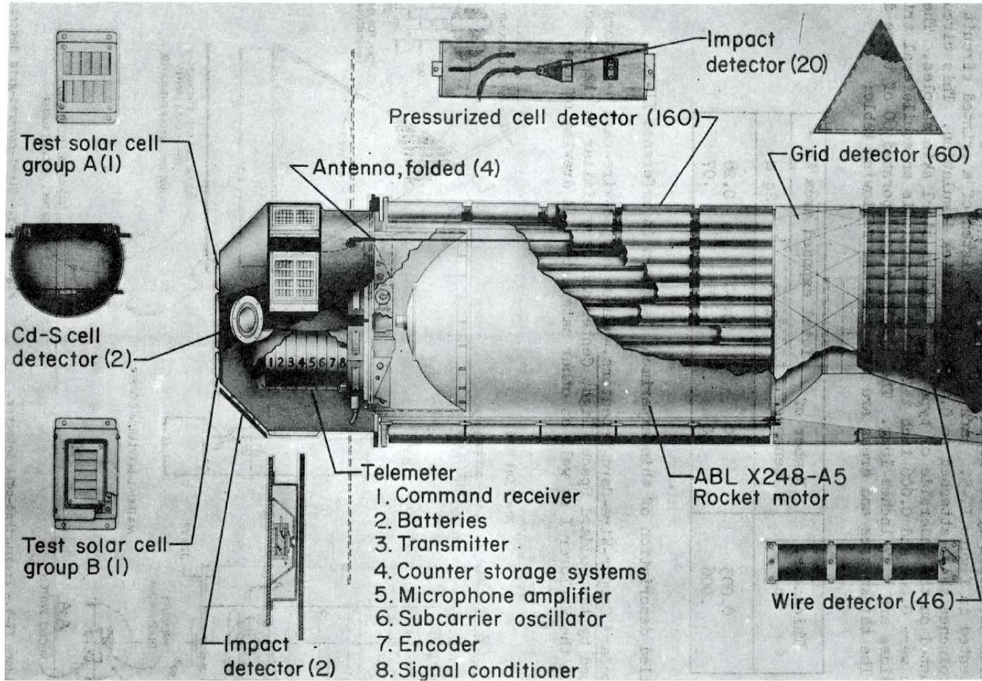
Explorer 13/16 Micrometeoroid Satellites
