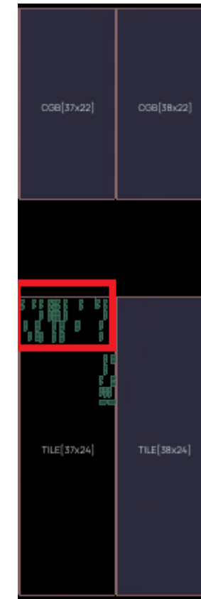
Adder mapped into LUT
