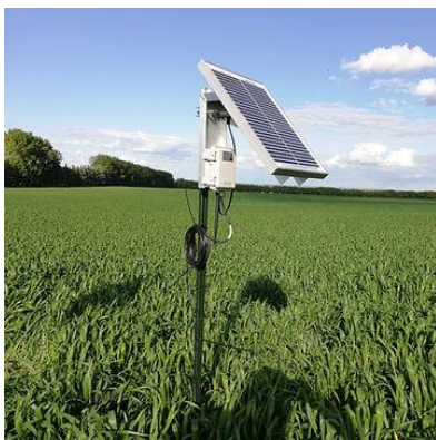
Figure 6 The current performance baseline for service B. It shows (left) An image of an in-situ sensor, (top) Data Allowance and (bottom) Upload/Download speeds, both compatible with LoRa-like and NB-IoT-like protocols.
