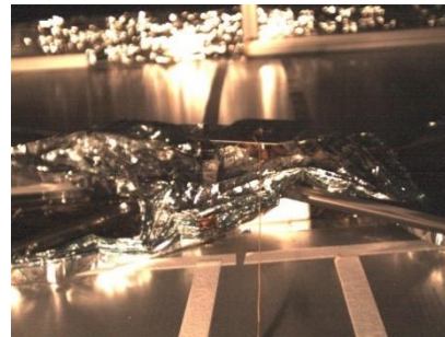
ADEO-N deployment in hot TVAC chamber
