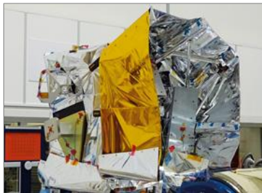
Thermal H/W (Radiators, Thermal Straps, MLI, etc)
