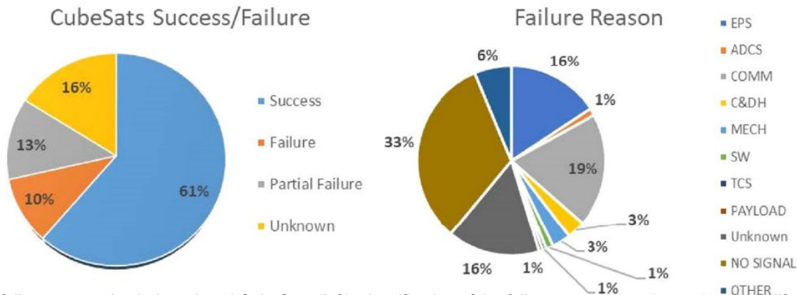
Figure 3: Rate of success/failure among the 672 analyzed CubeSats (left); classification of the failures per reason (center) and per lifetime (right) [3]
