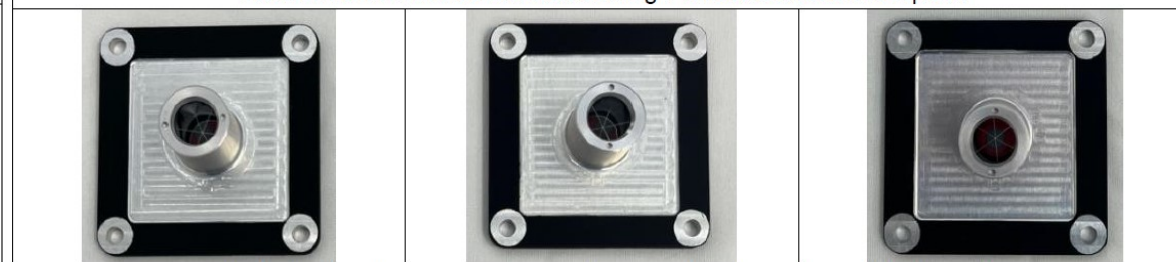
Trivalent chromium conversion coating + polyurethane based black paint
