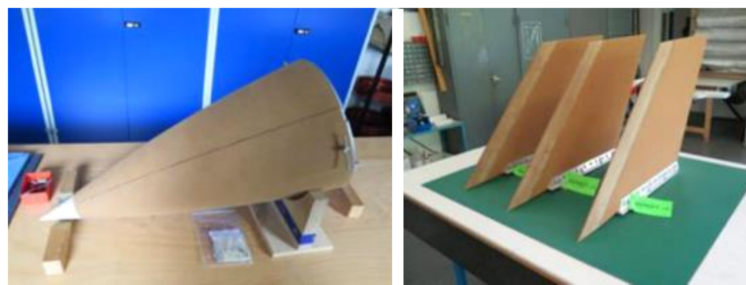
Application of cork-based thermal protection system (TPS) in primary and secondary launch vehicle structures [3]
