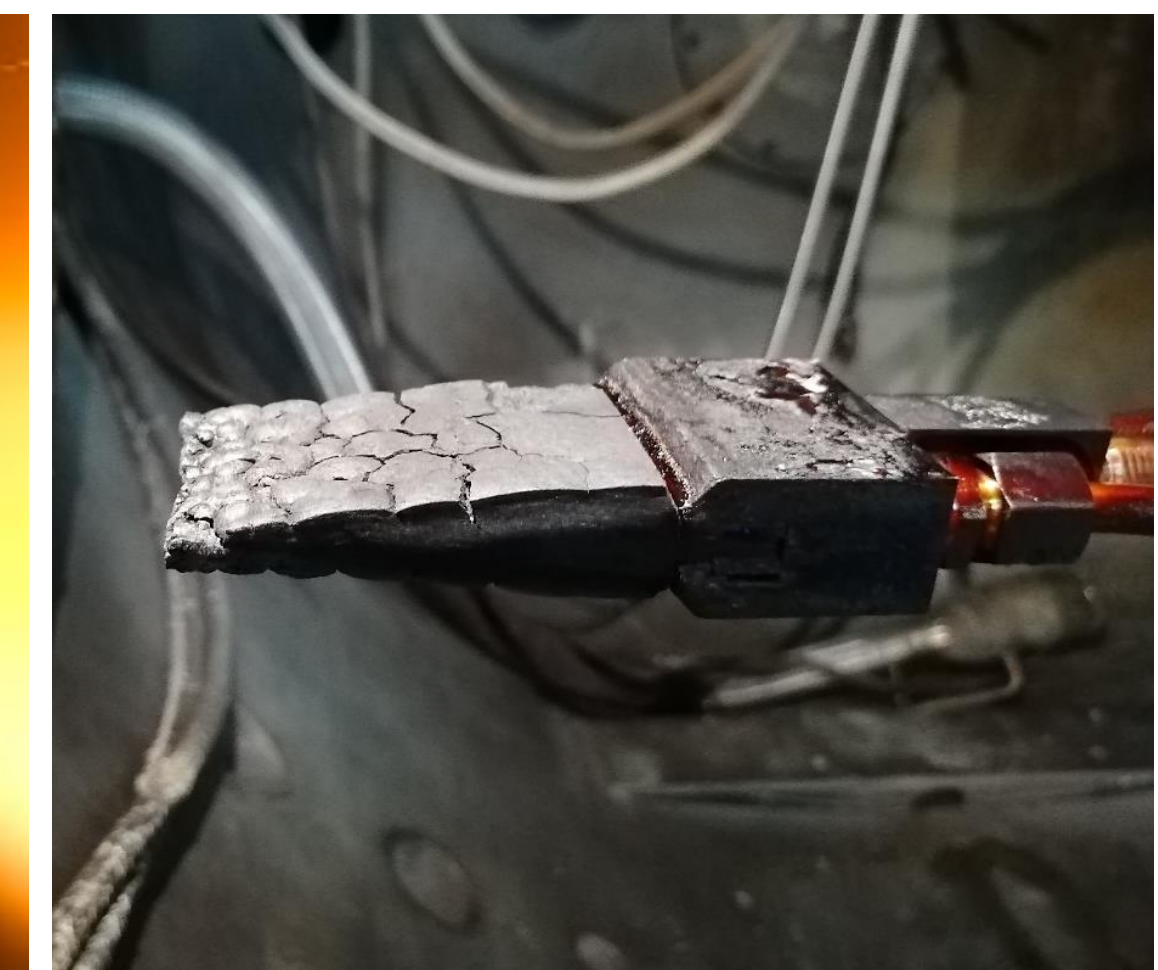
Carbonised test specimen after testing in L2K
