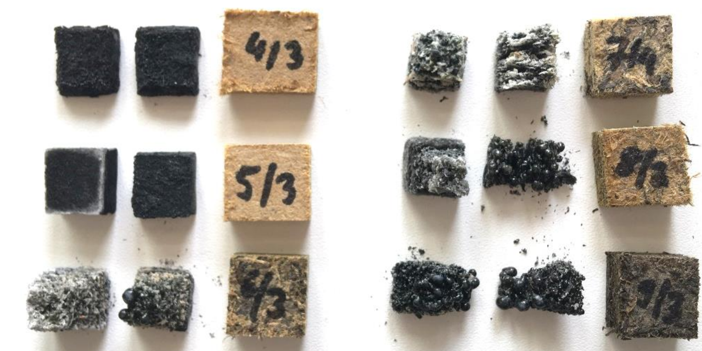
Test specimen of TPSea before and after TGA
