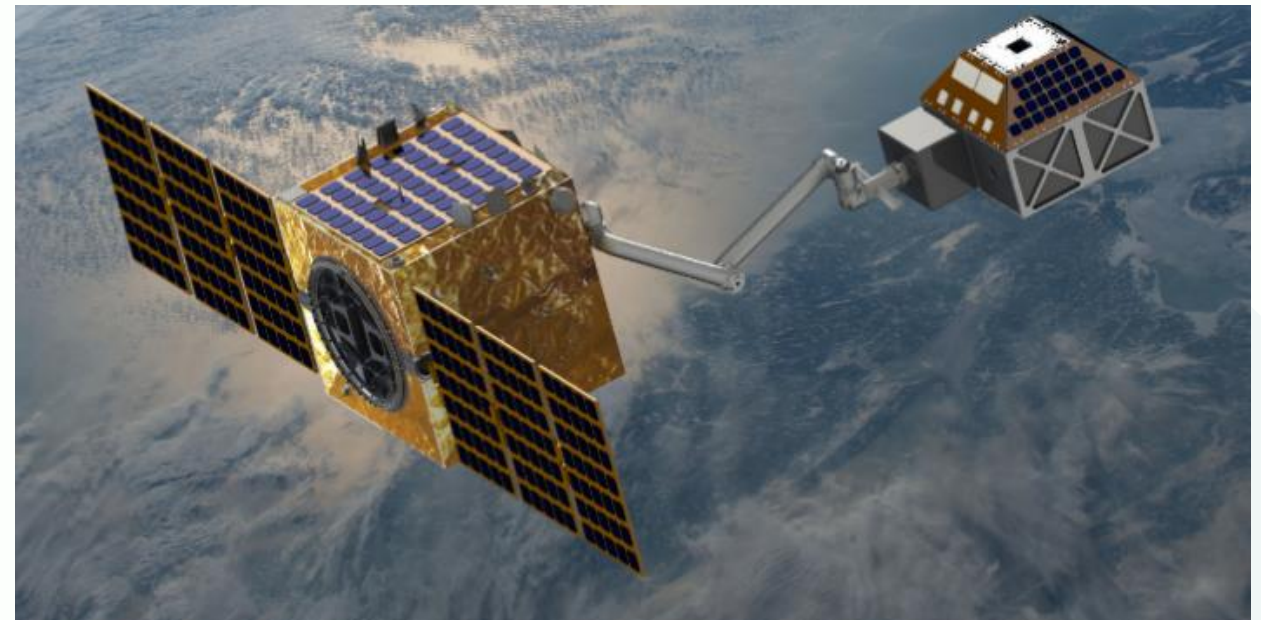
Fig. 9. A rendition of the ASUK servicer replacing a client unit
